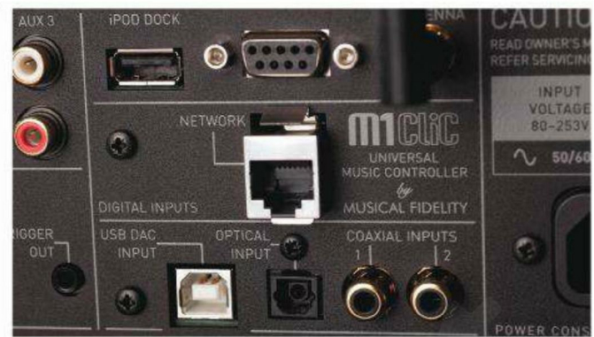
Ethernet, USB and iPod ports, as well as TosLink and coaxial S/PDIF inputs.
